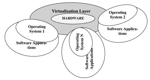
**Fig.1.** The Virtualization Layer provides a layer of abstraction between hardware and the applications
