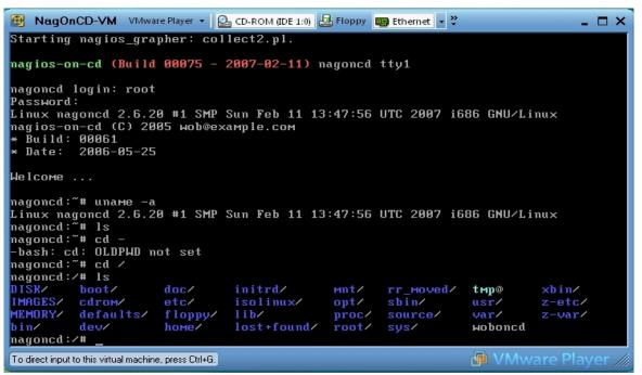
**Fig.5.** A Debian-based appliance running on the Windows<sup>™</sup> version of VMware Player
